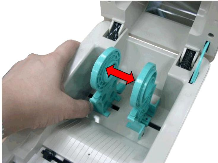
4. Place the roll between the holders and close them onto the core. Place the paper, printing side face up, through the media guides, media sensor and place the label leading edge onto the platen roller.
