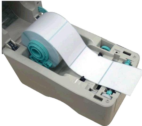
5. Move the media guides to fit the label width by turning the media guide adjuster knob.
