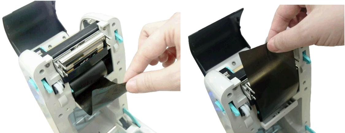
6. Stick the ribbon onto the ribbon rewind paper core.
