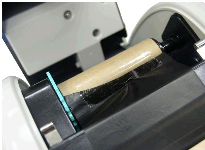
7. Turn the ribbon rewind gear until the ribbon plastic leader is thoroughly wound and the black section of the ribbon covers the print head. Close the ribbon access cover and the top cover.
