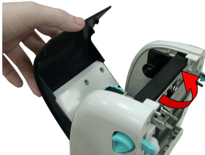
4. Insert the paper core right side onto the rewind hub. Align the notches on the left side and mount onto the spokes.
